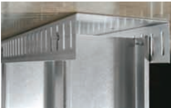
MaxTrak Slotted Deflection Track has slots in the legs to allow for vertical deflection.
