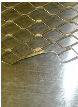
This illustration shows where the lath product has crimped on the ends due to cutter-tooling wear.
